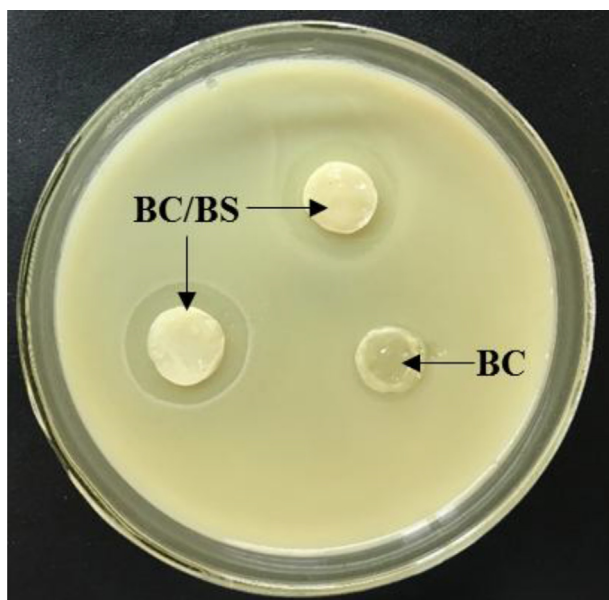
Fig. 7. Clear zone on skim milk agar around pure BC film and BC/BS biocomposite.
